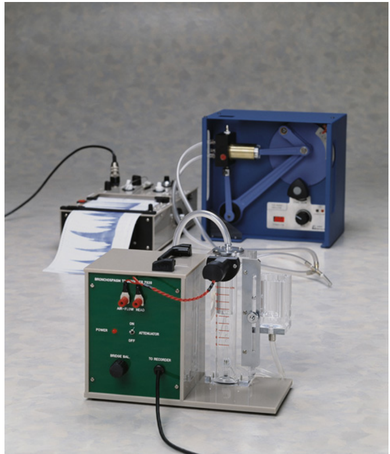
The picture shows a complete set-up for bronchodynamics studies which includes the Rodent ventilator 7025 and a pen recorder
